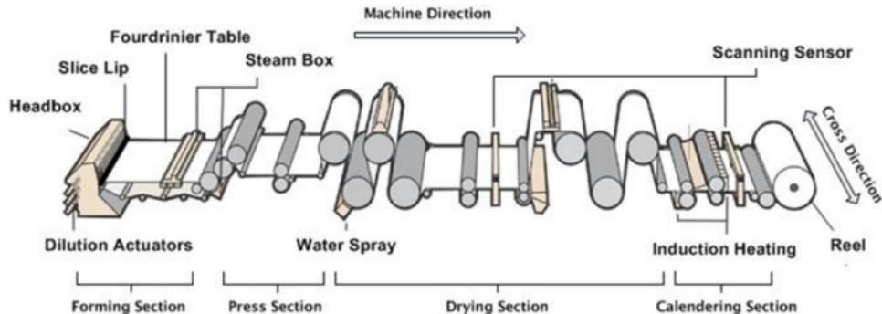
Source: Chu et.al. (2011), "Model Predictive Control and Optimization for Papermaking Process", doi: 10.5772/18535.
