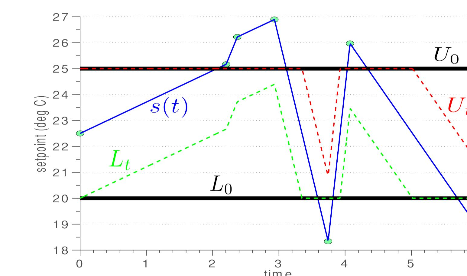
Fig. 3. Setpoint control with comfort range constraint to track optimal reference power trajectory.
