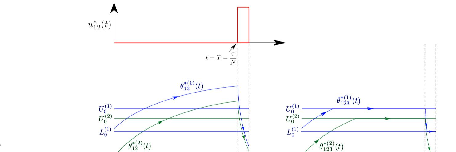
Fig. 9. Optimal control (top) and optimal temperature (state) trajectories (bottom)
