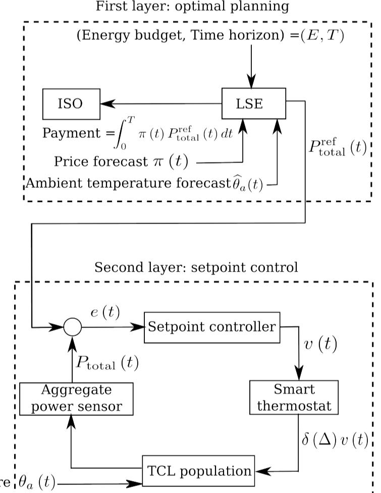
Fig. 2. Block diagram for the two layer control framework.
